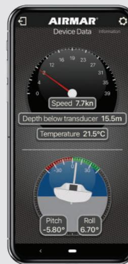
The Airmar CAST™ app is a mobile application that allows you to connect to your Airmar Smart™ TRIDUCER® multisensor. You can view data, adjust the outputs, program offsets and calibrate your sensor.
