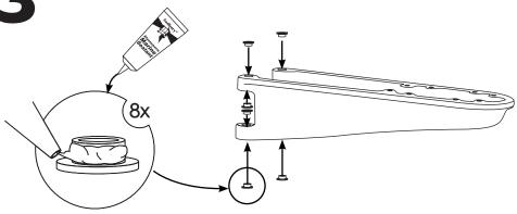
Once all shoulder washers are inserted attach the two mast mount feet.
