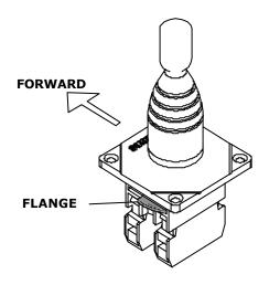
The joystick is anchored to the contact block by means of a snap-on flange. It should not be necessary to disconnect the joystick and the contact block for installation. If they have been disconnected, the joystick and the mounting plate have to be positioned into the contact block according to the drawing to get the correct port and starboard commands.
