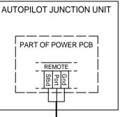
*Note: After installation, always check that correct direction of rudder movement is obtained. If not, reverse the red and the green wires!*
