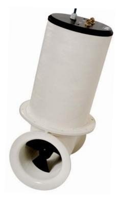
Details:12VProduct ref.:MPSPC812 / PODTypical boat size:32 - 51'Tunnel diameter (inside):185mmTunnel thickness:6 - 7mmNominal power voltage:12VControl system voltage:12V
