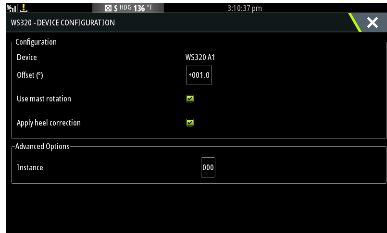
Example of configuration settings available via Device List (MFD display)
