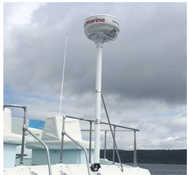
A hard anodized adjustable base with a water tight cable gland.
